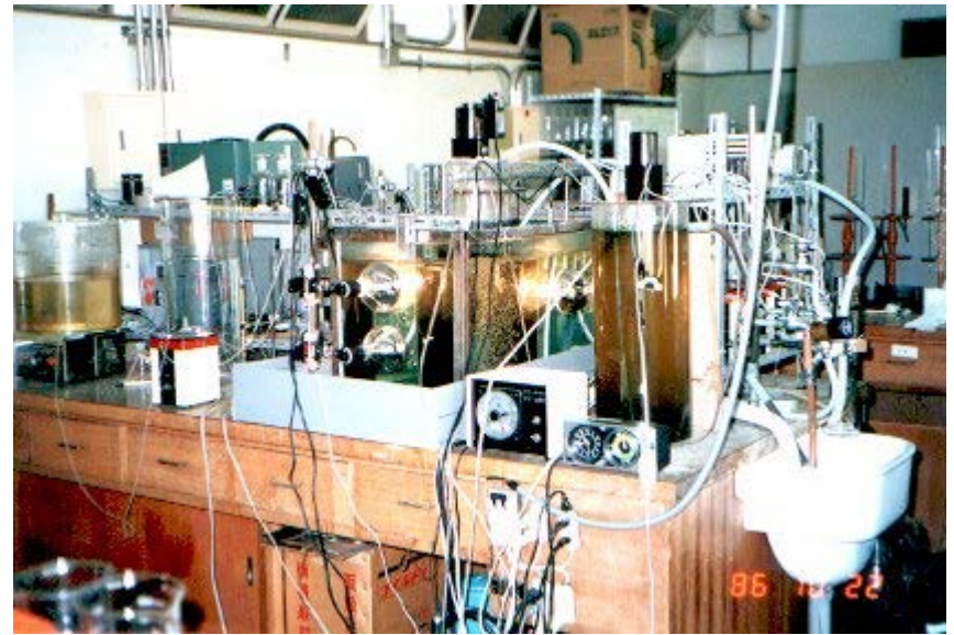
A full view of algal continuous-cultivation equipment with a nutrient salts feeder, illuminators, a separator which is set at the leftist side, and controllers.
